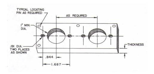
The above drawing shows the spacing and diameter of the leg location holes. The two standard 1151-M legs are inserted into these holes. To ensure that the welded stud is perpendicular to the work surface, a third leg, shortened by an amount equal to the template thickness, may be used in the weld gun. This leg is held in contact with the template during the weld cycle.
