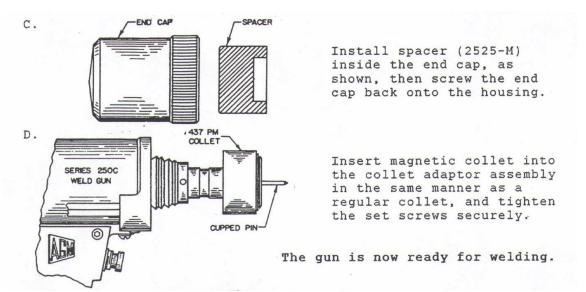
THIS SET UP IS FOR WELDING TO 22 GA. (.033") AND THICKER MATERIAL. DO NOT TRY TO WELD THROUGH PAINT OR RUST!
