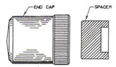
Install the 2525-M spacer inside the end cap,as shown, then screw the end cap back on the housing
